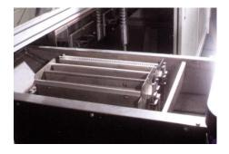
Solder Pot comes with Chip and Lambda Wave with the option of either Titanium or Ceramic Coated Cast Iron.
