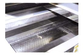
1800 to 2000mm of IR and convection preheat for even heating and better temperature slope.
